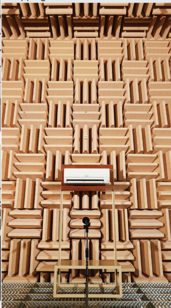
Anechoic Chamber Noise Test
